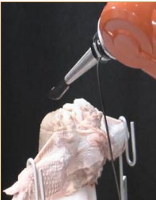
Initial work focused on developing a testcell to support studies on innovative automation cutting techniques. The cell constructed consists of a research robot, a variety of cutting end-effectors, a miniature force-torque sensor, and an array of digital cameras. In addition, the design team developed a computer model that incorporates measured cutting trajectories used by skilled workers to debone a chicken breast.
