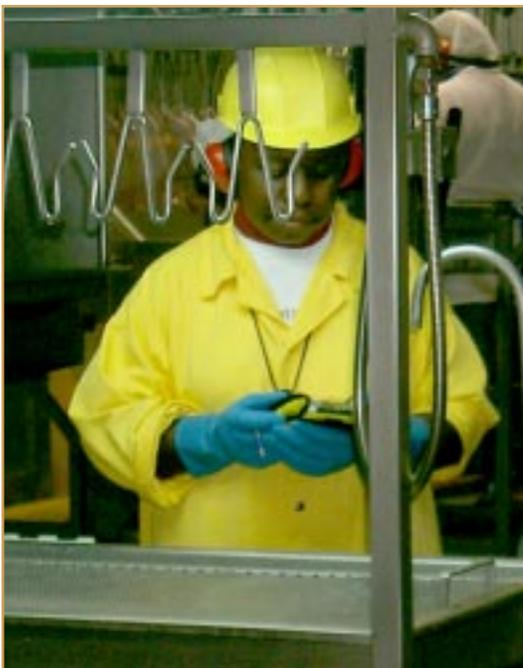
The Mobile Computing System project saw the installation and implementation of Tech's mobile electronic data-collection system in Cagle's poultry processing plant in Perry, Georgia. The data-collection system uses commercial hardware components, custom software, and a human-computer interface design to create a robust HACCP data-collection tool.
