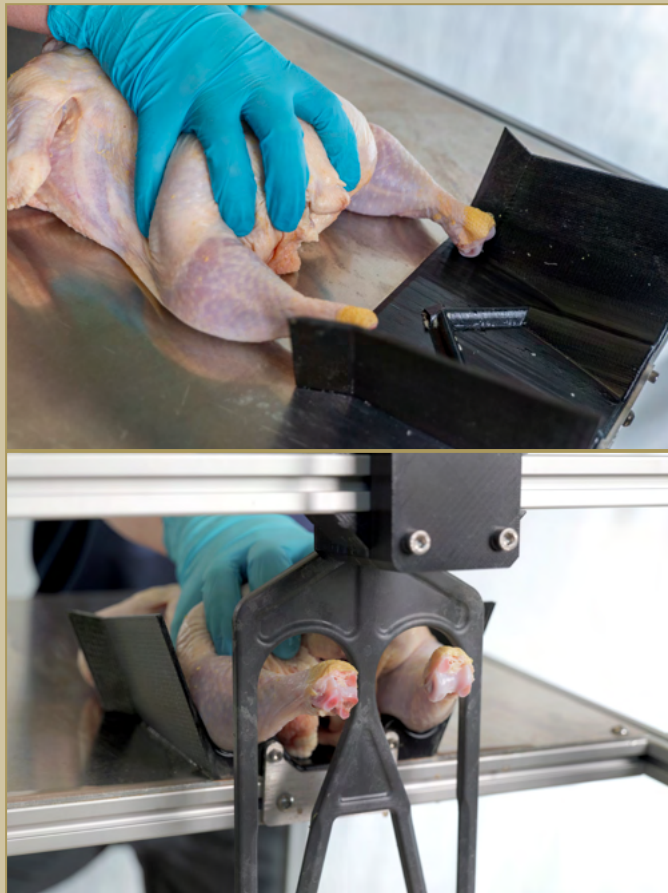
Demonstration of rehang mat aligning and singulating legs for shackling. Rather than hanging the bird by the legs, an operator simply slides the bird onto the specially designed mat positioned on a moving conveyor line. The line then raises and carries the product with it, greatly reducing the need for strenuous lifting.
